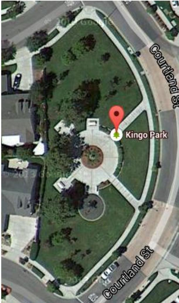
Remove turf from parkways (station #1 and #2). Convert to drip for existing trees and new shrubs. Install DG along parkway. Remove turf behind fountain between concrete and wall (station # 9). Convert station #4 to MP3500 rotors. Total potential water savings of up to **39,413 gallons per month** minus whatever emitters are used for new plants and existing trees.
